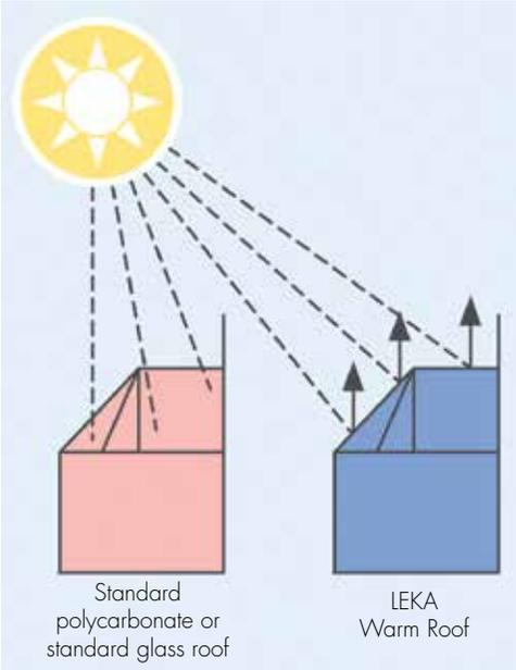
The LEKA Warm Roof has been designed and engineered to offer you so much more. It is a truly lightweight tiled conservatory roof with an overall U-Value of just  $0.15\text{W/m}^2\text{K}$ . This makes the LEKA Warm Roof one of the most lightweight and energy efficient roofs on the market today and offers the perfect balance between energy efficiency and comfortable living.
